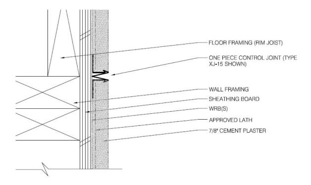
The single-piece control joint can accommodate small amounts of anticipated movement and stress, such as shrinkage of dimensional wood framing on low to midrise construction. Significant movement (greater than 1/4 inch) would necessitate a two-piece expansion joint. A second control joint may be placed at the top of rim joist.
