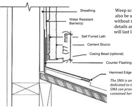
Weep screeds, casing beads and step flashings may also be used, but may not allow for re-roofing without removing of a section of stucco. These details assume the stucco was installed correctly and will last longer than the roofing or decking material.
