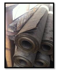
tensile strength. The asphaltic products had another major benefit for stucco, they wrinkle when wet. The wet scratch coat causes the paper to wrinkle and form shallow channels. When the plaster dries, the asphaltic paper releases substantially from the dry cement. This results in a weep or drainage plane behind the stucco.
